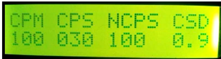
Figure 14: Display showing compressions per minute (CPM), compressions per set (CPS), number of compression sets (NCPS) and compression set delay (CSD).
