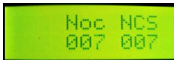
Figure 13: Display of number of compressions (Noc) and number of compressions set (NCS)
