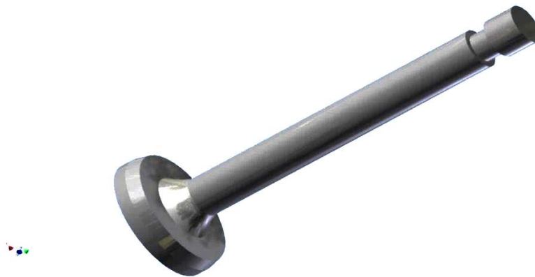
Fig.3: 3D Modelling of Poppet Valve
