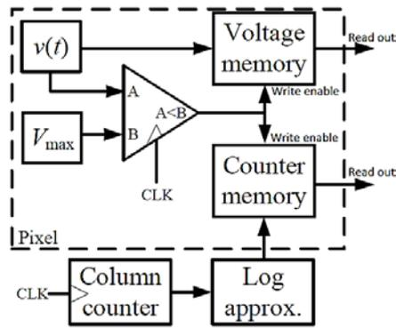
Fig. 2. A block diagram of the proposed sensor's counter-memory architecture.
