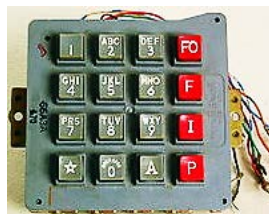
Figure 3: DTMF Keypad matrix [3].
