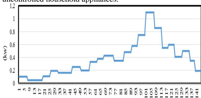
FIGURE 3- UNCONTROLLED ENERGY CONSUMPTION LOAD CURVE OF HOME APPLIANCES.
