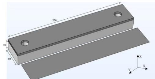
Fig. 2. Test specimen laminated by SiFe sheets.
