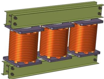
Fig. 1. Transformer model for structure analysis.
