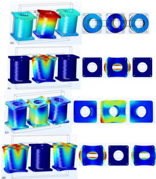
Fig. 5. The first four winding-related modes at (a) 320Hz, (b) 398Hz, (c) 401Hz, and (d) 468Hz.
