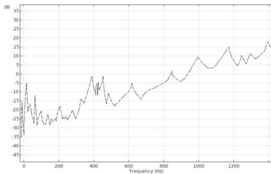
Fig. 3. Spatially averaged FRF of the power transformer.
