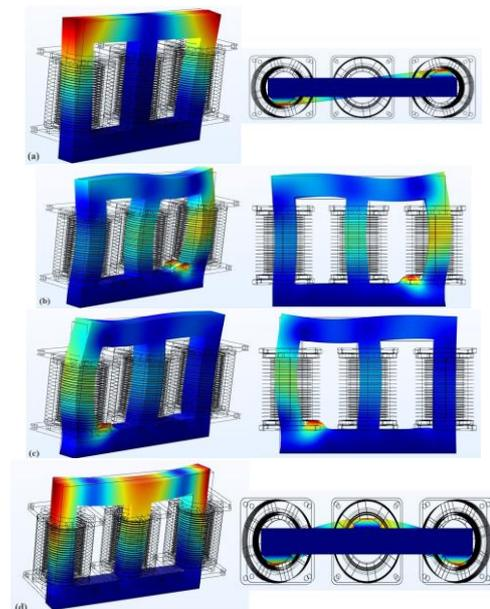
Fig. 4. The first four core-related modes at (a) 32Hz, (b) 56Hz, (c) 79Hz, and (d) 105Hz.
