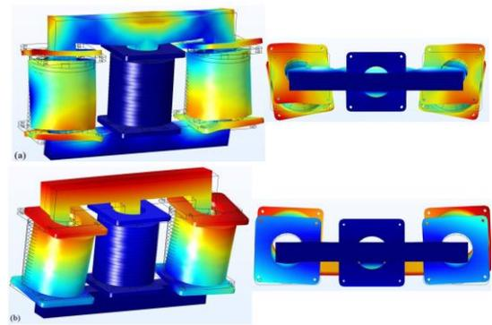
Fig. 6. The first two core-winding coupled modes at (a) 14Hz, and (b) 21Hz.
