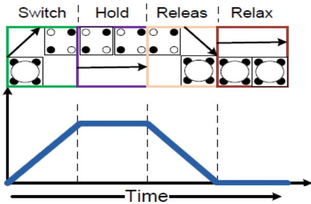
Fig. 2. QCA clocking with different phases [31].
