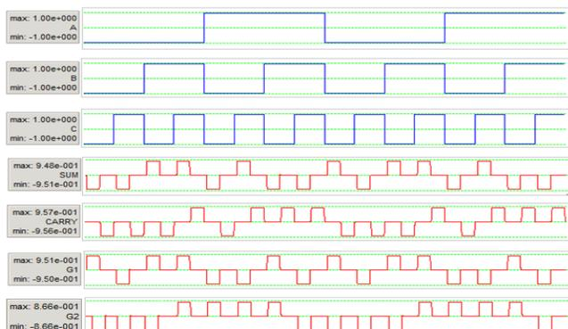
Fig. 12. Display of the input - output waveforms for the proposed QCA 1-bit reversible full adder.
