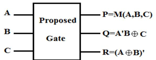
Fig. 5. Schematic of the proposed reversible gate Block diagram.
