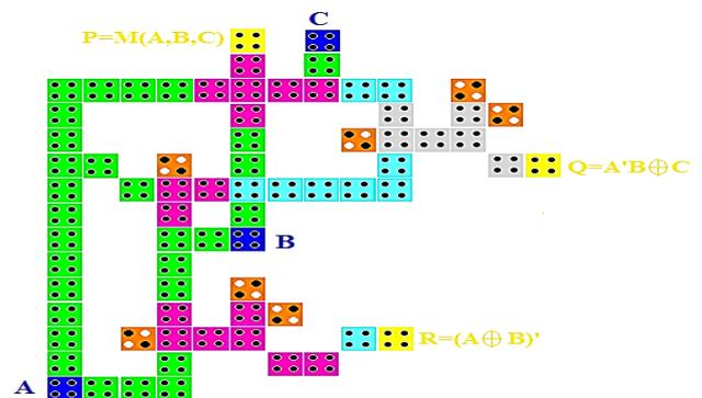
Fig. 6. QCA implementation of the new  $3 \times 3$  reversible gate.
