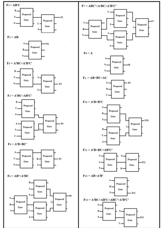
Fig. 7. Implementation of All 13 standard logical functions using the new proposed reversible gate.
