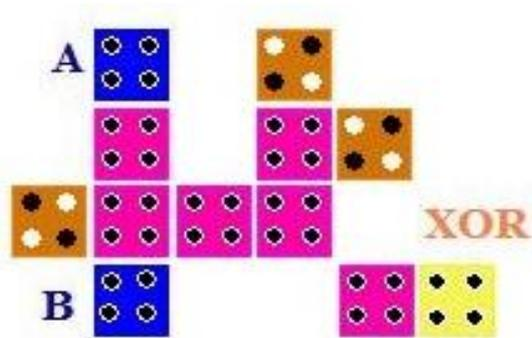
Fig. 4. QCA layout of the improved proposed XOR structure.
