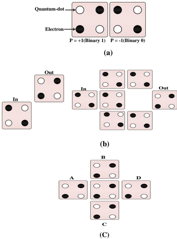
Fig. 1. Main QCA structures (a) QCA cell, (b) Different type of Inverter gate, (c) 3-input majority gate.
