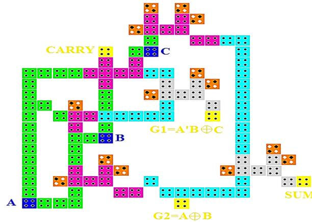
Fig. 10. Display of the QCA layout for the new reversible full adder.
