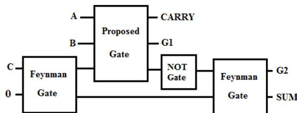
Fig. 9. Schematic of the proposed reversible full adder.
