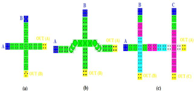
Fig. 3. Different methods of wire-crossing: (a) Coplanar rotated cells, (b) Multilayer, (c) Coplanar clocking based [32].
