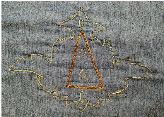
Fig. 1. Embroidered fabric with conductive thread.
