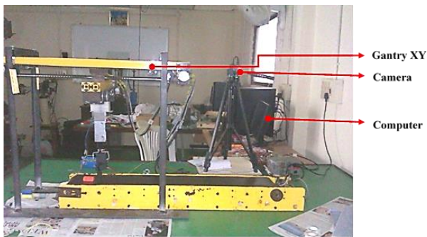
Fig. 17 Object sorting robot using machine vision inspection system
