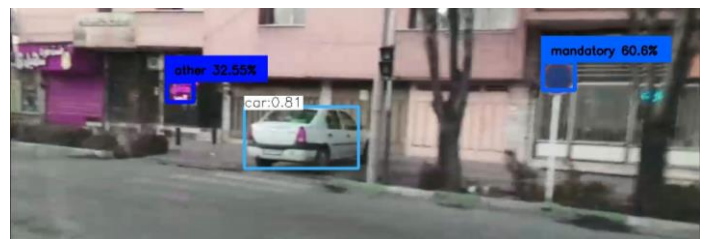
Fig. 5. Detection Error due to the low threshold level of the correct detection.
