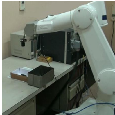
Figure 1: Robotic system for picking randomly oriented texture less cylindrical objects in multiple layers.
