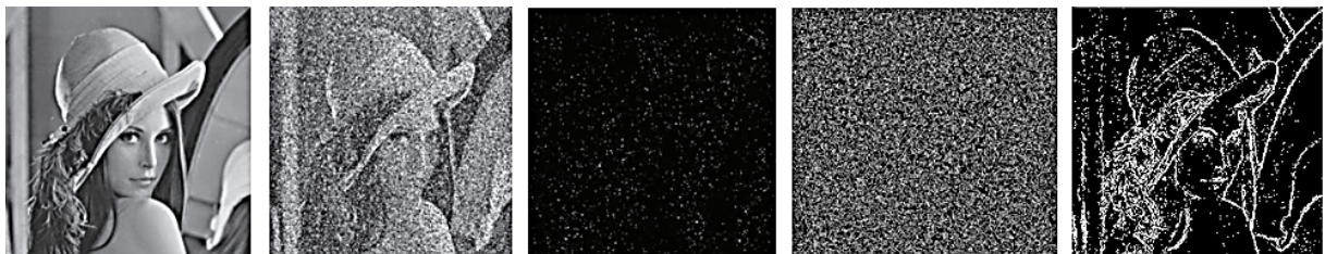
Figure 7: Comparison of the proposed edge detector with the Sobel and the canny edge detectors. From left to right: Original, Noisy, Sobel, Canny Proposed method [18].
